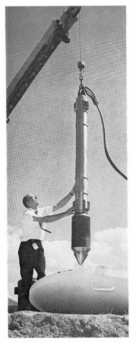
PROTOTYPE USO package was guided into 169-foot deep borehole in Coyote Test Field by Dean Gladow (9233).
